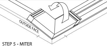
HOOK OUTSIDE FACE OF MITER ASSEMBLY ONTO CONTINUOUS CLEAT AND ROTATE INTO PLACE.
