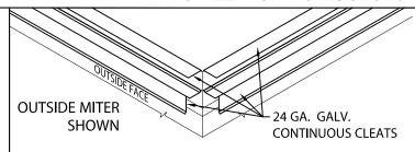
STEP 1 - CONTINUOUS CLEATS AT CORNERS PLACE OUTSIDE CONTINUOUS CLEATS ON BOTH SIDES OF CORNER AND TWO INSIDE CONTINUOUS CLEATS ON BOTH SIDES. DO NOT FASTEN CLEATS AT THIS TIME.
