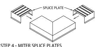
REMOVE RELEASE PAPER FROM TOP OF FACTORY APPLIED SEALANT STRIPS, INSTALL THE SPLICE PLATES INTO EACH **END OF THE MITER AS SHOWN**
